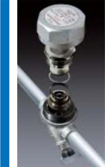
Disc-type steam traps often fail from wear due to the repetitive impact of the valve disc against the valve seat. With the A3N's replaceable module, these parts can easily be replaced as a single unit, reducing replacement time and maintenance costs.
