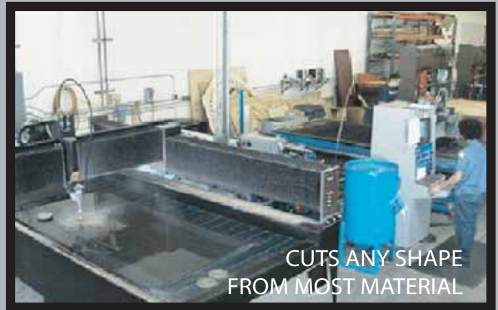
5'x10' bed, computer controlled, dual water jets in Cerritos, CA and Pascagoula, MS.
