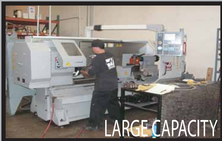
CNC lathe featuring 28" OD X 72" length capacity with twin 24" chucks and 7" through bore.
