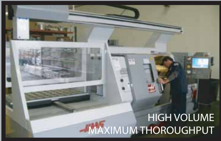
CNC Lathe w/Automatic Parts Loader featuring 10" OD X 20" length capacity
