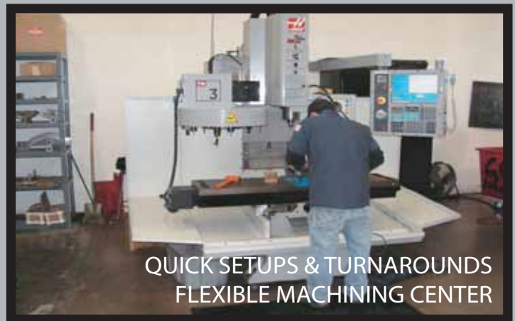
40" X 20" CNC mill with 20 station tool changer and 3 axis capability
