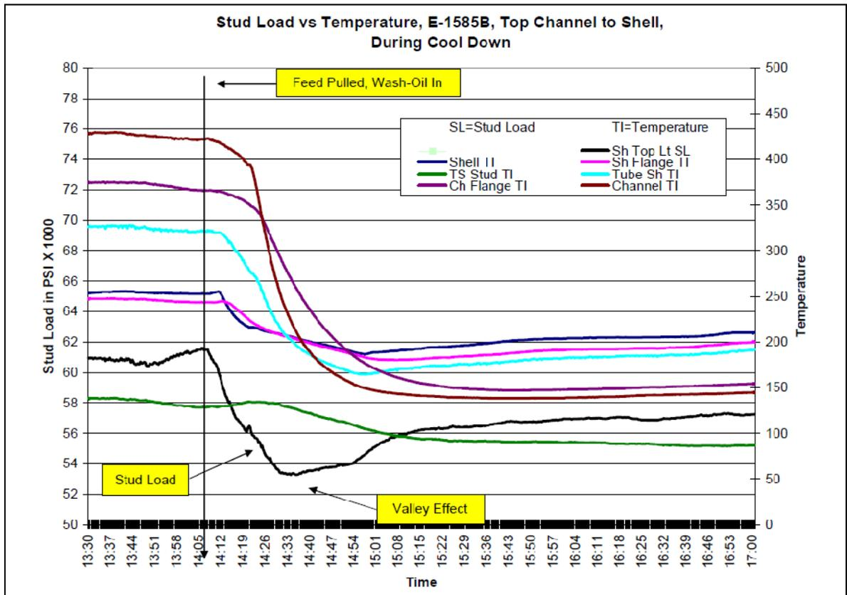
Clearly, the practice of insulating flanges tips the scale in favor of developing more leaks. So as a general rule, flanges should not be insulated.
