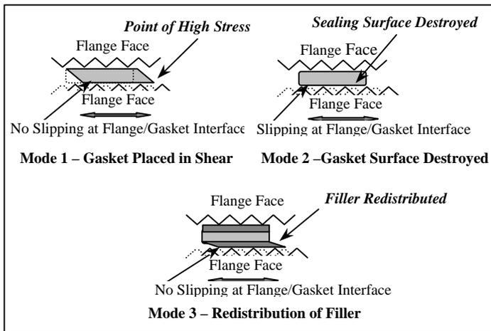
**Figure 5 – Gasket Failure Modes due to Radial Movement**
