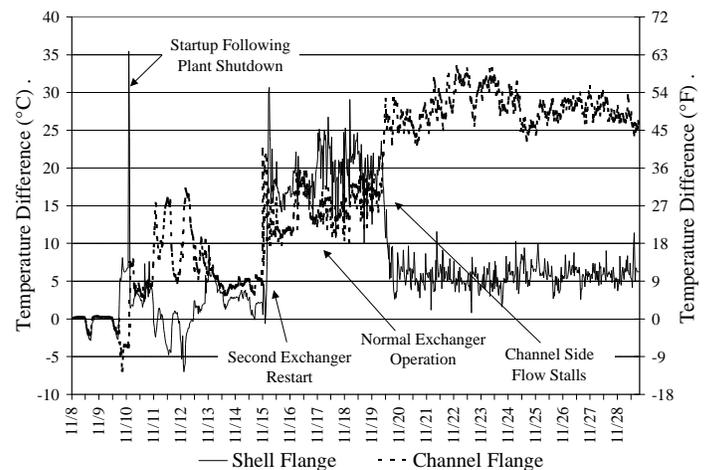
Figure 3 – Difference between tubesheet and flange temperatures for 21 days of operation
