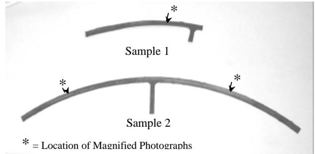
**Figure 6 – Double Jacketed Gasket Samples**
