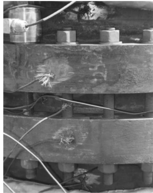
Figure 2 – Thermocouple Placement
