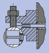
Designed for ASME B16.5 or ASME B16.47 with spin fit outer guide ring for thermal expansion.
