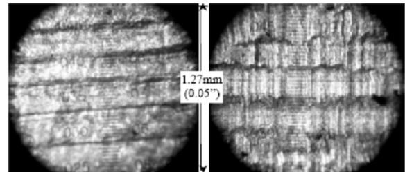
The picture on the left shows a gasket firmly clamped by the flanges. This sample had failed when stress fatigue split the inside radius of the Double Jacketed gasket. The picture on the right shows striations as the flange scraped across the surface of the gasket.
