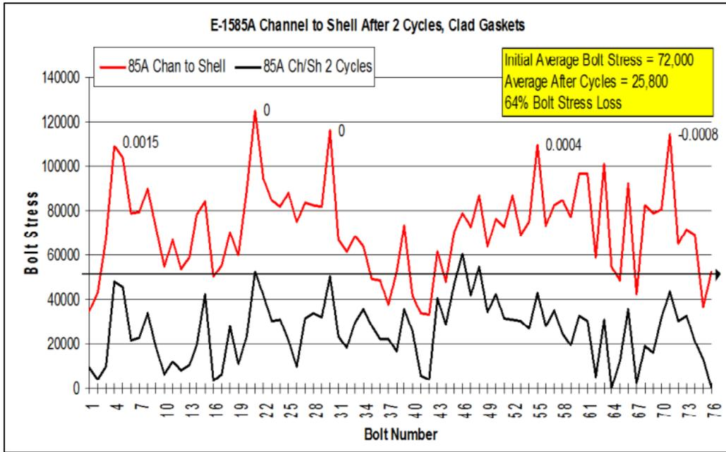
The data in red shows the initial stud load on each of the 76 studs – averaging 72,000-psi stud stress. The data in black shows the residual stud stress just two thermal cycles later, when the unit was leaking profusely. The average stud stress had dropped 64% to just 25,800-psi.
