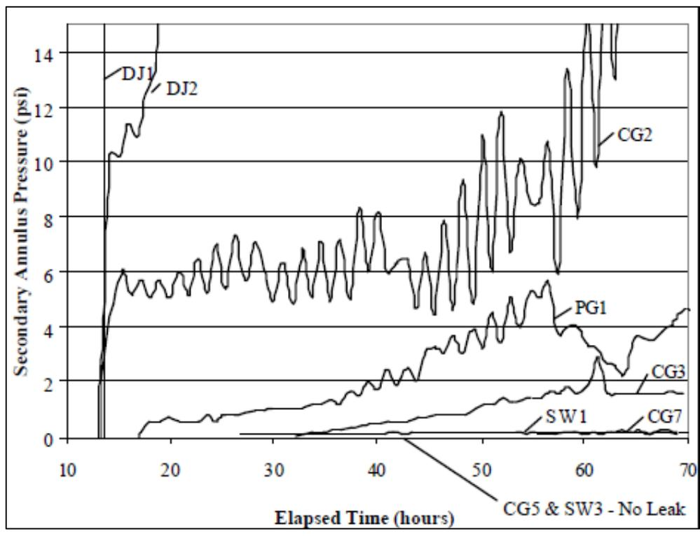
The testing needed to optimize the corrugated gasket was conducted in the field at a Southern California refinery. Various tests were designed to determine the optimal:
