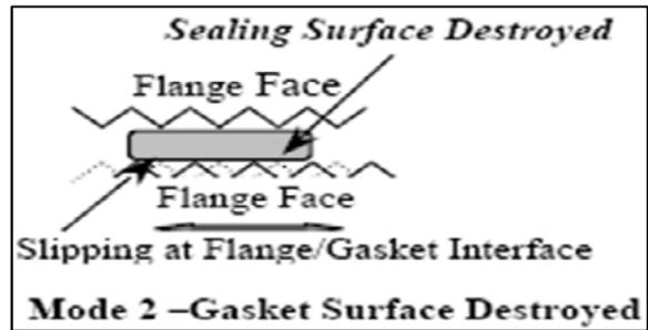
A photo micrographic inspection of the failed gasket samples confirmed both of these modes of failure.
