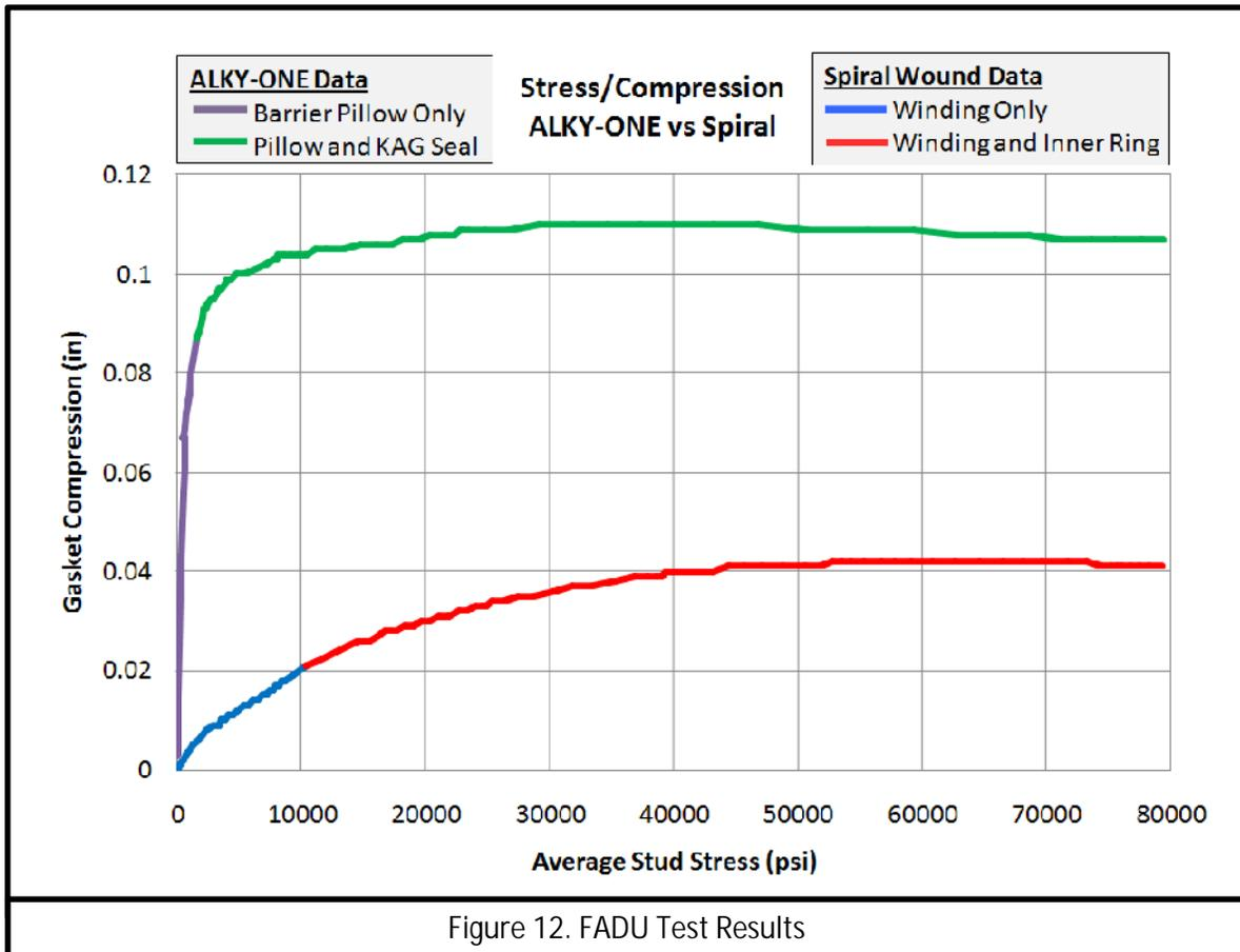
Figure 12. FADU Test Results
