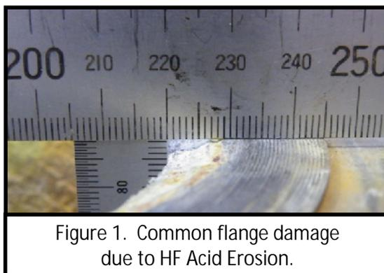
Figure 1. Common flange damage due to HF Acid Erosion.
