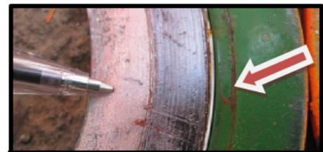
Figure 2. Flange Imprint on Used Gasket
