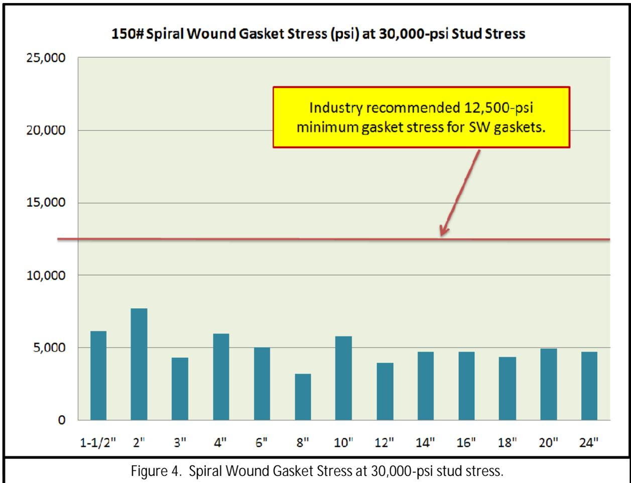
Figure 4. Spiral Wound Gasket Stress at 30,000-psi stud stress.
