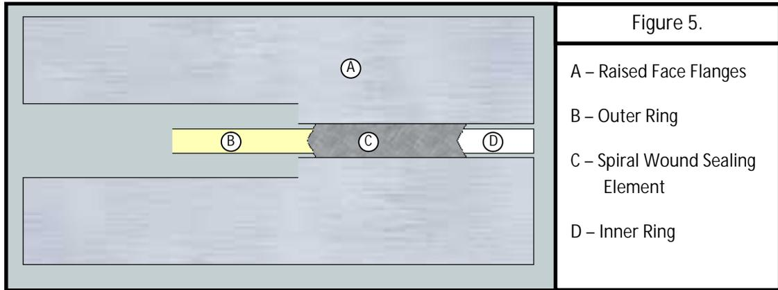
The inner ring of a standard spiralwound gasket is the same thickness (1/8") as the outer ring. The outer ring is intended both to center the gaskets in the bolt circle and to provide a compression limiting stop to the flanges, while the inner ring protects against inward buckling of the winding and serves as a gap-filler on the ID of the flanges.
